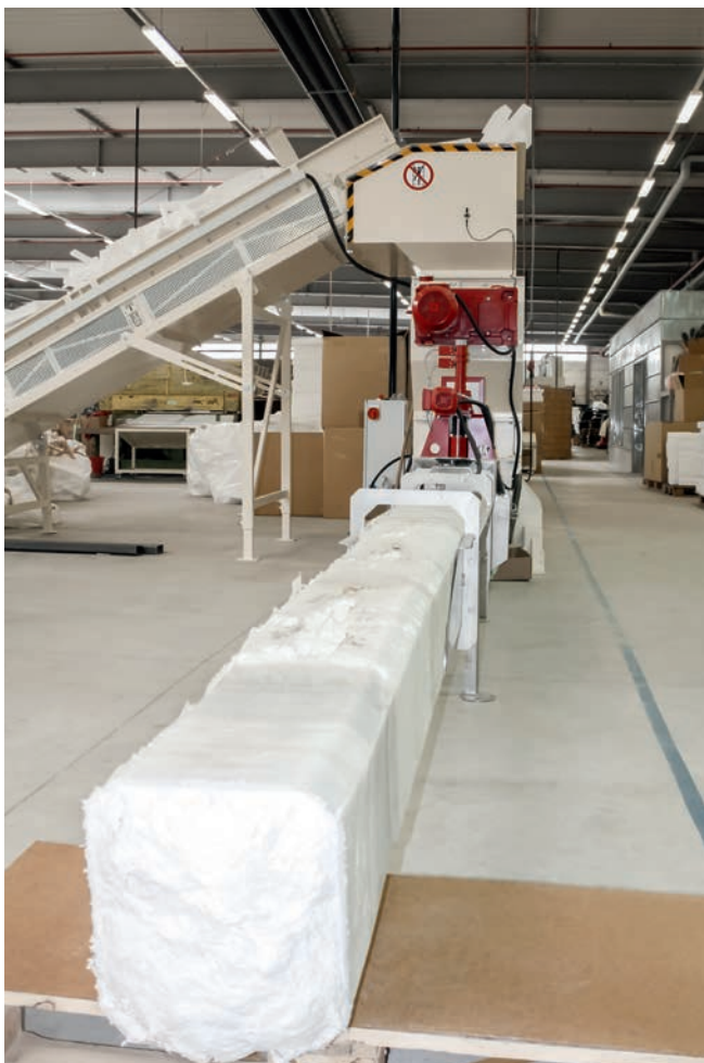
The foam waste that occurs in production is pressed and then recycled.
