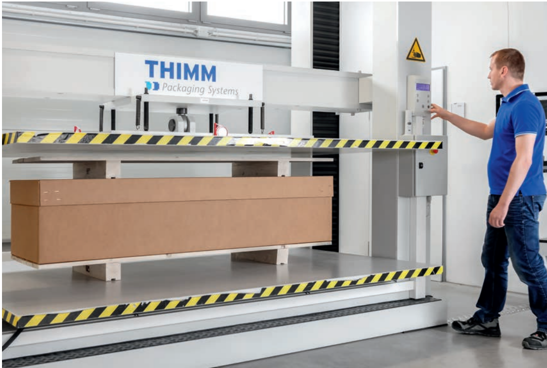
Large load carriers for industry are subject to a quality test.
