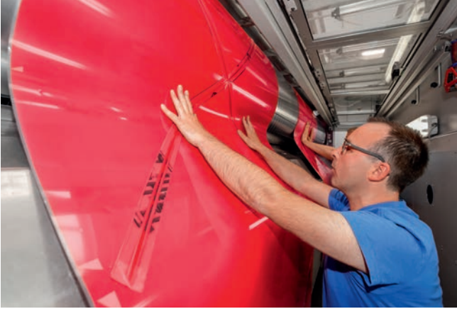
Set-up of an inking unit.
